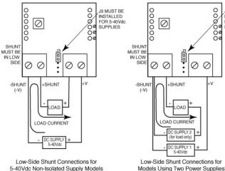
Operation with 36 to 75Vdc Power: As shipped, all models rated operating supply range is -5 to +40Vdc. However, DLA20-DGA models can be user configured for 36 to 75Vdc operation by removing (opening) jumper J3. Also, all models - including those that have been modified for 36-75Vdc operation can only be connected in low-side, grounded-shunt applications.
